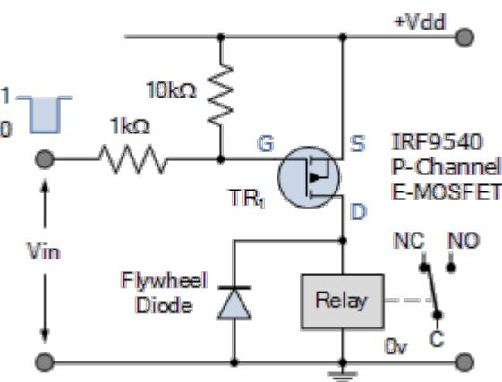
In this configuration, the P-channels Source terminal is connected to +Vdd and the Drain terminal is connected to ground via the relays coil. When a HIGH voltage level is applied to the Gate, the P-channel MOSFET will be turned "OFF". The turned "OFF" E-MOSFET will have a very high channel resistance and acts nearly like an open circuit.
