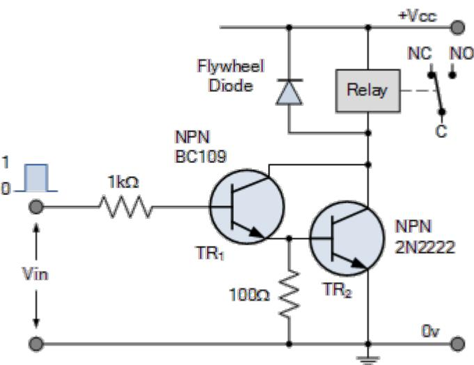
If two individual transistors are configured as a Darlington switching pair, then a small value resistor (100 to 1,000Ω's) is usually placed between the Base and Emitter of the main switching transistor, TR2 to ensure that it turns fully OFF. Again a flywheel diode is used to protect TR2 from the back emf generated when the relay coil is de-energised.
