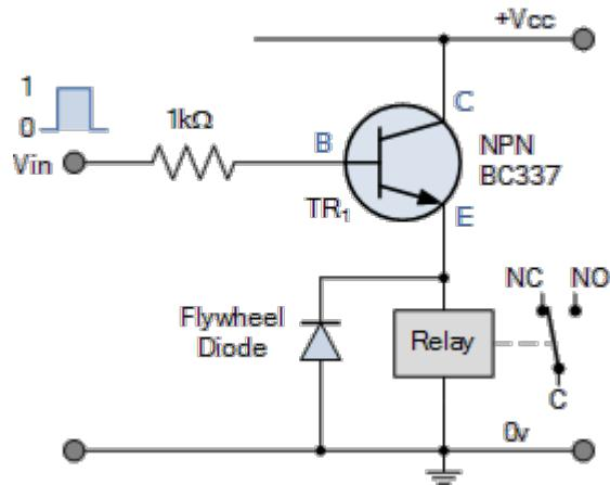
The Common Collector, or Emitter Follower configuration is very useful for impedance matching applications because of the very high input impedance, in the region of hundreds of thousands of Ohms while having a relatively low output impedance to switch the relays coil. As with the previous NPN relay switch circuit, switching occurs by applying a positive current to
