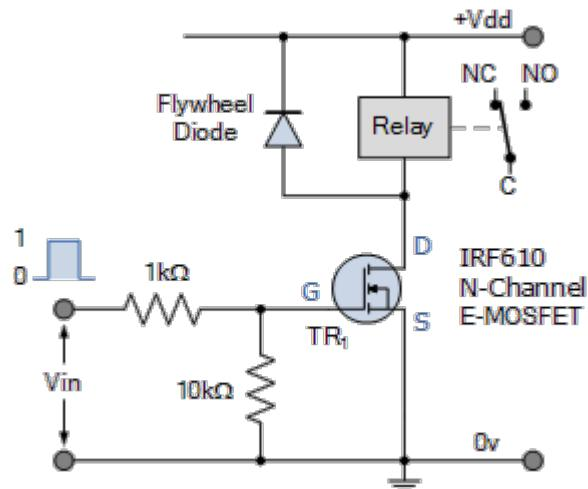
The above MOSFET relay switch circuit is connected in a common-source configuration. With zero voltage input, LOW condition, the value of  $V_{GS}$ , there is insufficient Gate drive to open the channel and the transistor is “OFF”. But when  $V_{GS}$  is increased above the MOSFETs lower threshold voltage  $V_T$ , the channel opens, current flows and the relay coil is operated.
