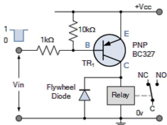
We have seen that either an NPN bipolar transistor or an PNP bipolar transistor can operate as a switch for relay switching, or any other load for that matter. But that there are two different conditions that need to be understood as the current flows in two different directions.
