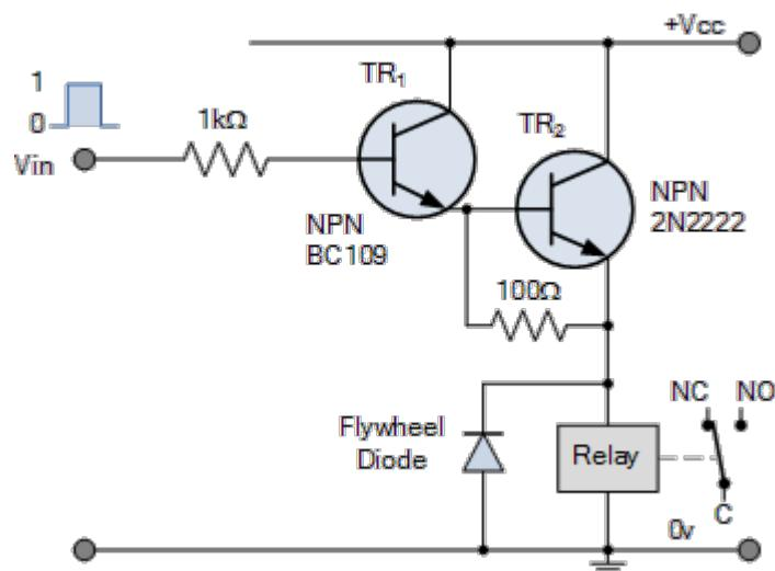
The Common Emitter Darlington relay switch circuit is useful to provide current gain and power gain with the voltage gain approximately equal to unity. Another important characteristic of this type of Emitter Follower circuit is that it has a high input impedance and a low output impedance, which make it ideal for impedance matching to large relay coils.
