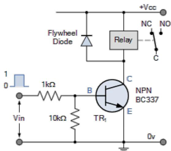
Note that the relay coil is not only an electromagnet but it is also an inductor. When power is applied to the coil due to the switching action of the transistor, a maximum current will flow as a result of the DC resistance of the coil as defined by Ohms Law, ( $I = V/R$ ). Some of this electrical energy is stored within the relay coil's magnetic field.
